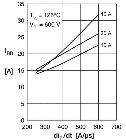
Fig. 3 Typ. peak reverse current  $I_{RRM}$  versus  $di_F/dt$
