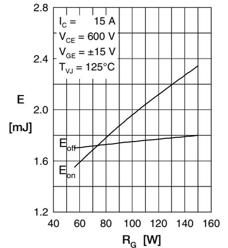
Fig. 6 Typ. switching energy versus gate resistance
