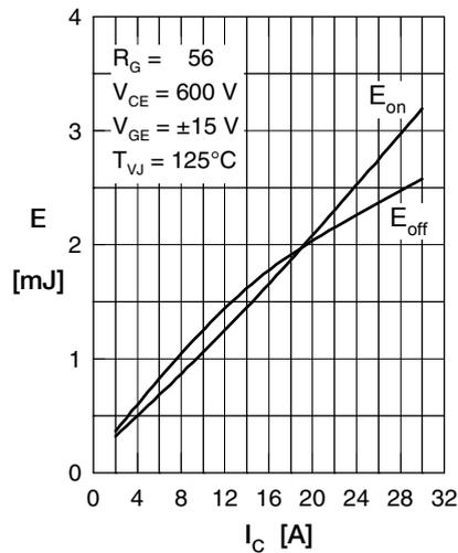
Fig. 5 Typ. switching energy versus collector current
