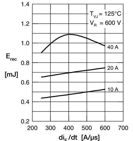
Fig. 6 Typ. recovery energy  $E_{rec}$  versus  $di/dt$
