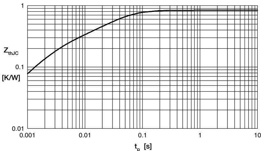
Fig. 7 Typ. transient thermal impedance junction to case
