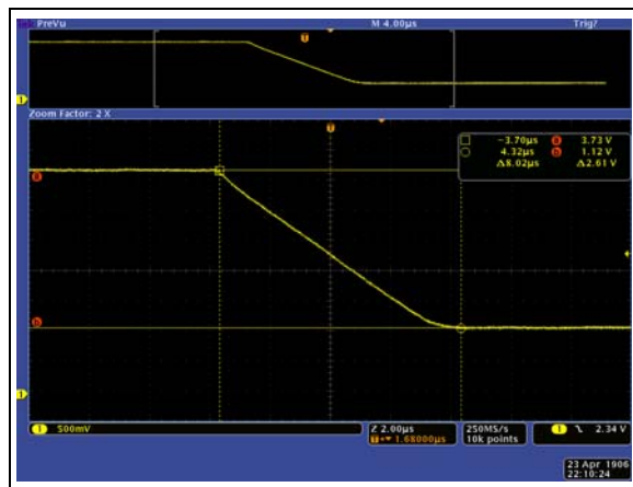
FIGURE 2-39: Half-Scale Settling Time (30h to 10h), V_{DD} = 5.0\text{V} , V_{REF} = 5.0\text{V} , R_L = 5\text{k}\Omega , C_L = 200\text{pF} (Time scale = 2\text{ }\mu\text{s} / \text{div} ).
