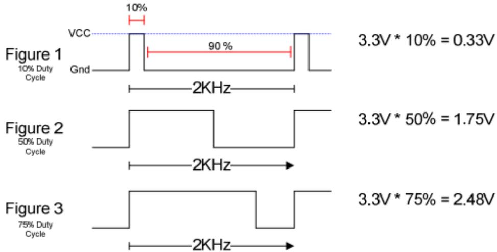
The way that this works is that when voltage is being applied, the motor is driven by the changing magnetic forces. When voltage is stopped, momentum causes the motor to continue spinning a while. At a high enough frequency, this process of powering and coasting enables the motor to achieve a smooth rotation that can easily be controlled through digital logic.
