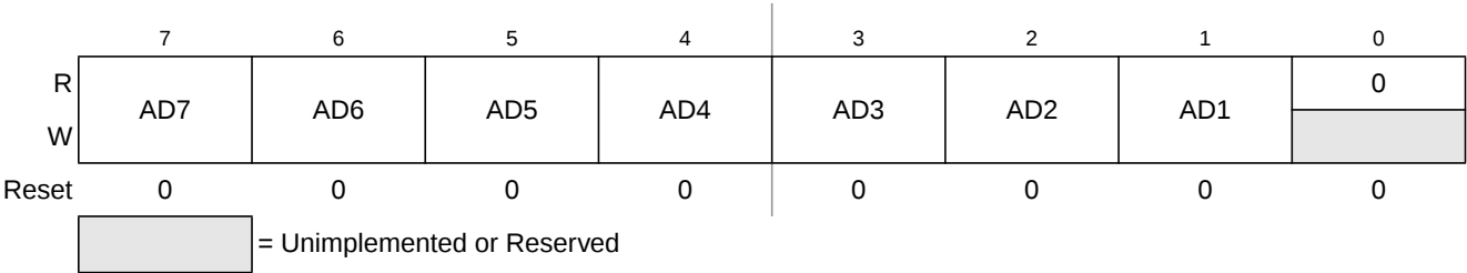
Figure 11-3. IIC Address Register (IICA)
