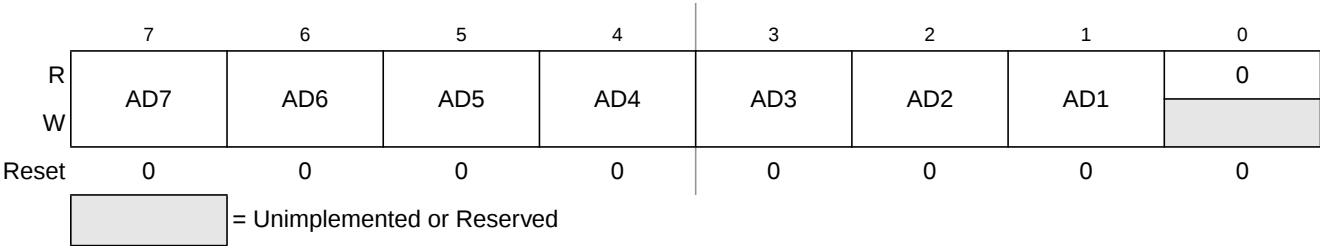
Figure 11-3. IIC Address Register (IICA)
