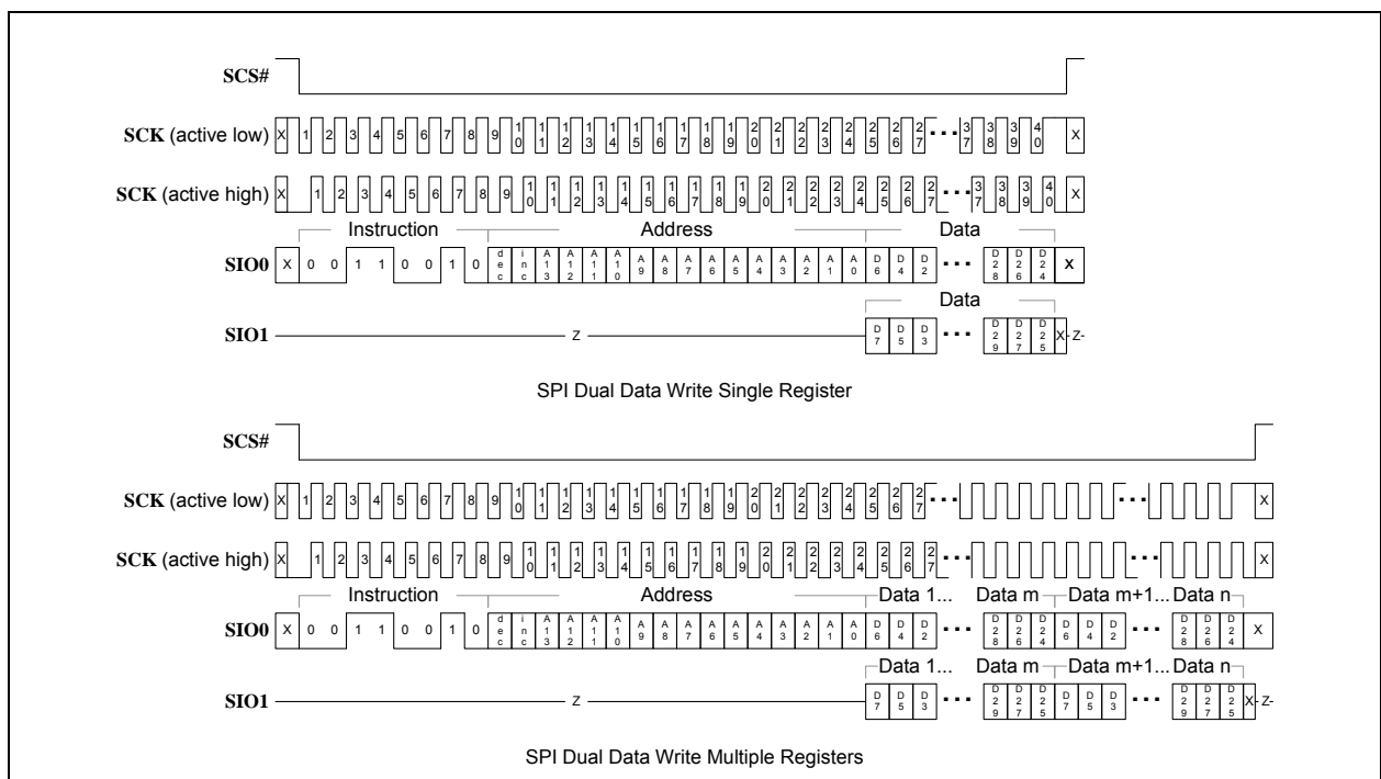
FIGURE 10-13: SPI DUAL DATA WRITE
