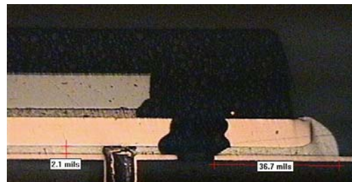
81% Paste Coverage, Encroached Via, 2.1 mil Standoff
