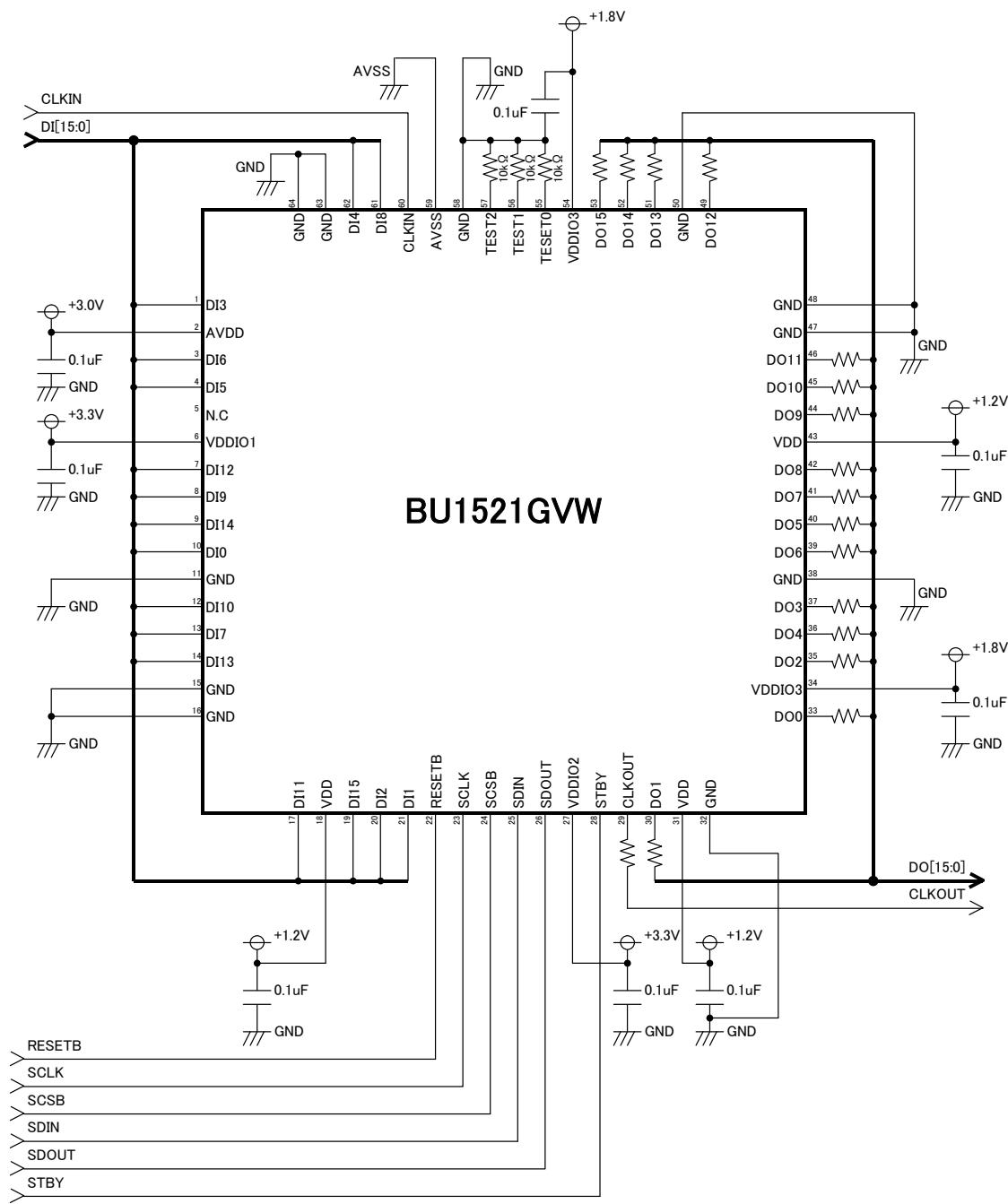
Note 1) Adjust the output damping resistance for CLKOUT and DO [15:0] with the line load.
