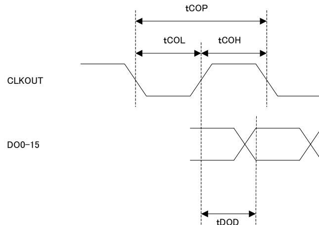
Fig. 3 Image Data Output Timing
