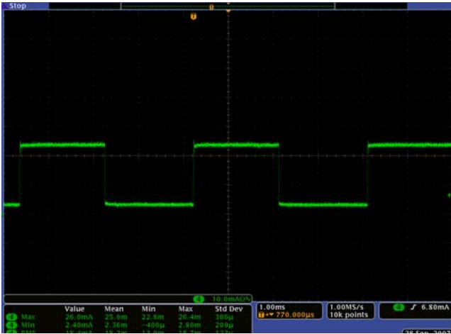
FIGURE 13. I_{LED} AT 50% PWM DIMMING
