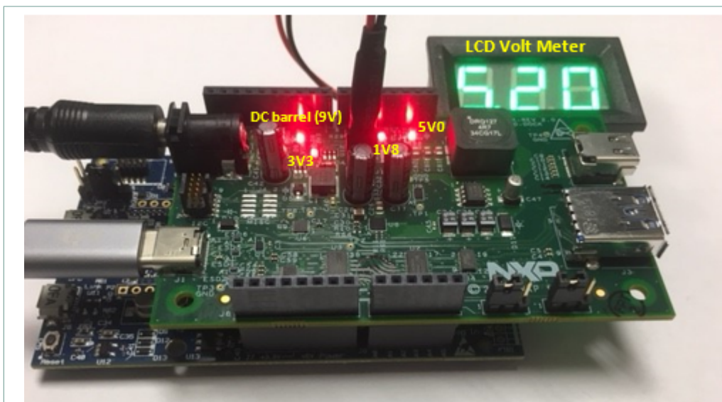
Figure 10. Shield 2 dock board control and LED indication
