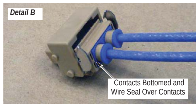
Mating Face of Plug Connector
