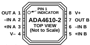
Figure 5. ADA4610-2 Pin Configuration, 8-Lead LFCSP_VD (CP Suffix)
