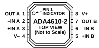
Figure 5. ADA4610-2 Pin Configuration, 8-Lead LFCSP_VD (CP Suffix)
