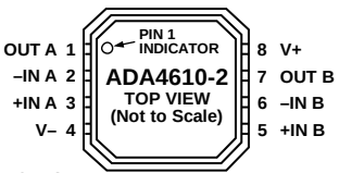
Figure 5. ADA4610-2 Pin Configuration, 8-Lead LFCSP_VD (CP Suffix)
