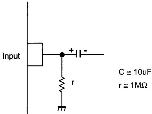
This IC requires 0.1μF capacitor between INPUT and GND, 1MΩ resistance between INPUT and GND for clamp type input at mute mode.
