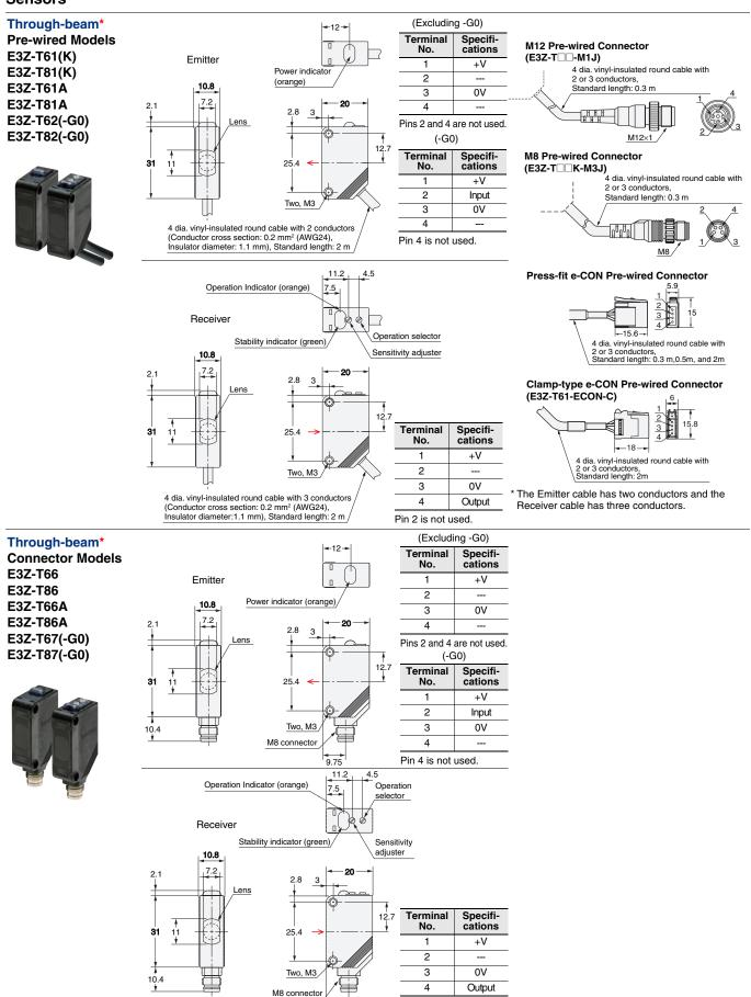
\* Models numbers for Through-beam Sensors (E3Z-T —) are for sets that include both the Emitter and Receiver. The model number of the Emitter is expressed by adding "-L" to the set model number (example: E3Z-T61-L 2M), the model number of the Receiver, by adding "-D" (example: E3Z-T61-D 2M.) Refer to Ordering Information to confirm model numbers for Emitter and Receivers.
