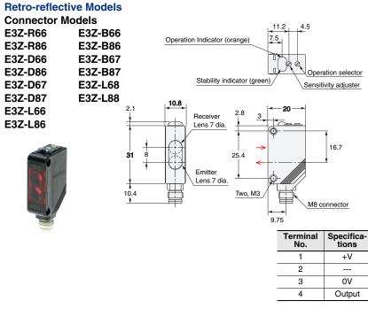
Note: The lens for the E3Z-D1/D6/L1/B is red. The lens for the E3Z-D2/D7 is black.
