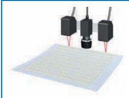
Inspecting Glass Heights (Autofocus)
