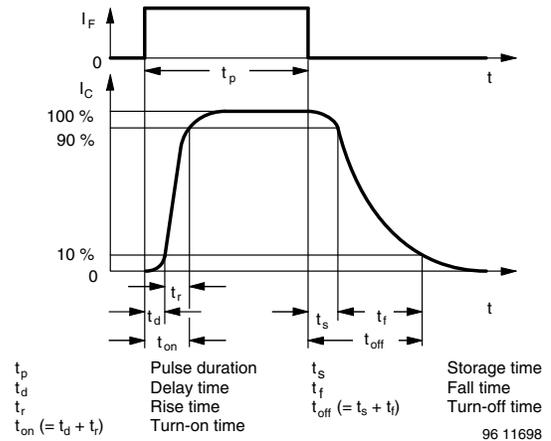
Fig. 3 - Switching Times
