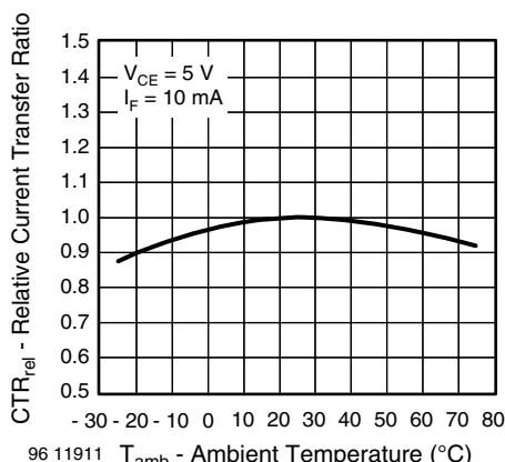
Fig. 6 - Relative Current Transfer Ratio vs. Ambient Temperature
