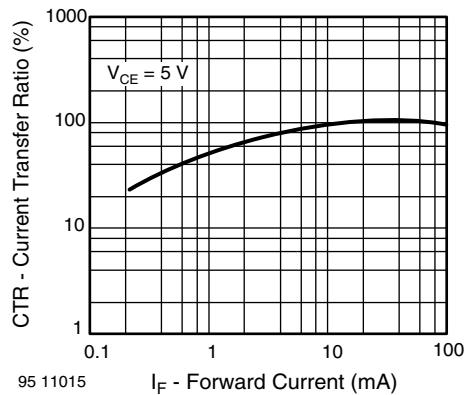
Fig. 11 - Current Transfer Ratio vs. Forward Current
