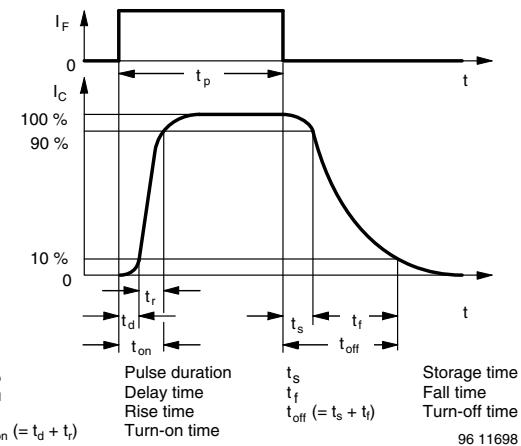
Fig. 3 - Switching Times
