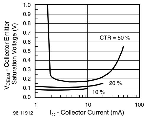
Fig. 10 - Collector Emitter Saturation Voltage vs.
