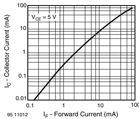
Fig. 8 - Collector Current vs. Forward Current
