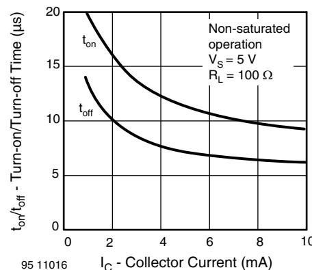
Fig. 13 - Turn-on/Turn-off Time vs. Collector Current
