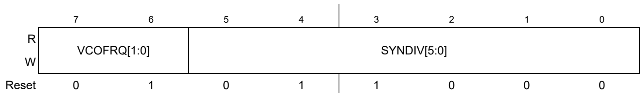
Figure 8-5. S12CPMU_UHV_V7 Synthesizer Register (CPMUSYNR)
