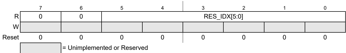
Figure 9-24. ADC Result Index Register (ADCRIDX)
