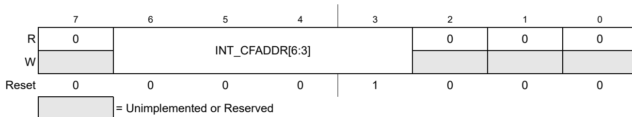
Figure 5-4. Interrupt Configuration Address Register (INT_CFADDR)
