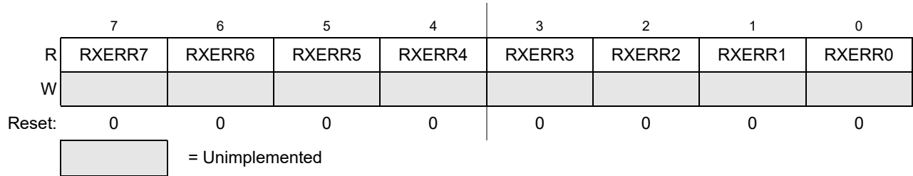
Figure 18-18. MSCAN Receive Error Counter (CANRXERR)
