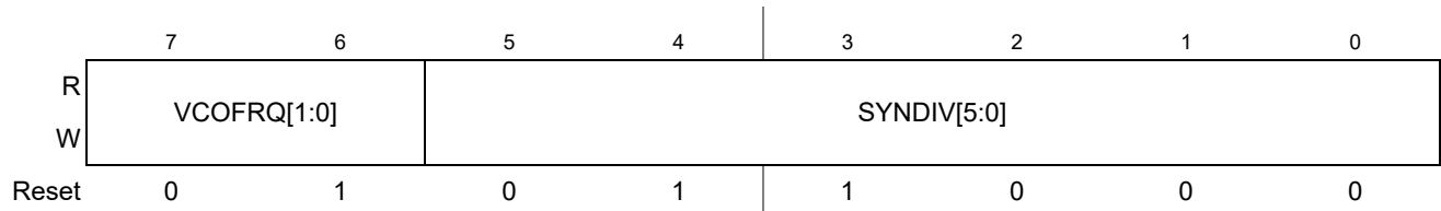
Figure 8-5. S12CPMU_UHV_V7 Synthesizer Register (CPMUSYNR)
