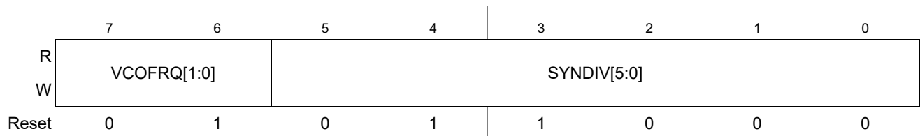
Figure 8-5. S12CPMU_UHV_V7 Synthesizer Register (CPMUSYNR)
