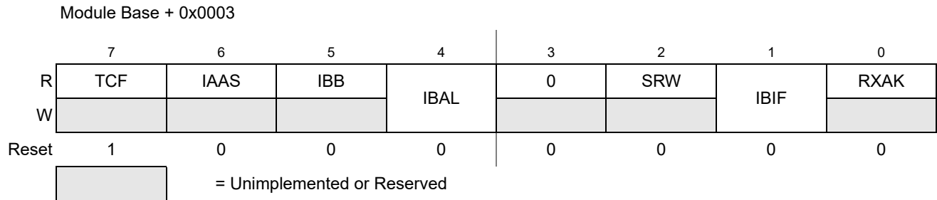
Figure 16-7. IIC Bus Status Register (IBSR)
