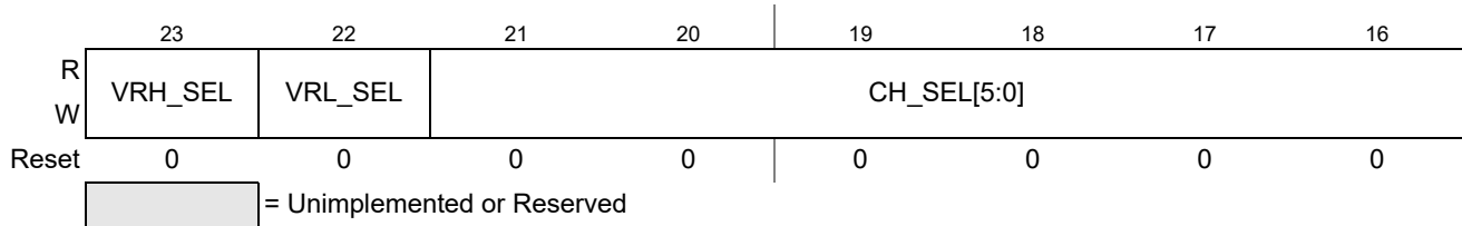
Figure 9-19. ADC Command Register 1 (ADCCMD_1)
