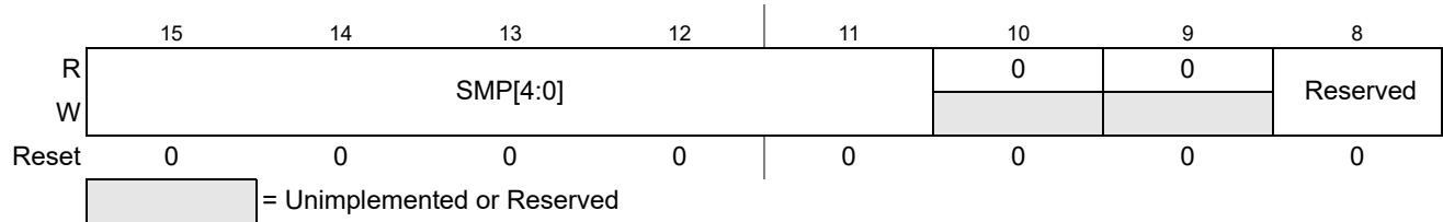
Figure 9-20. ADC Command Register 2 (ADCCMD_2)
