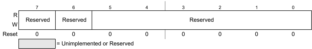
Figure 9-21. ADC Command Register 3 (ADCCMD_3)
