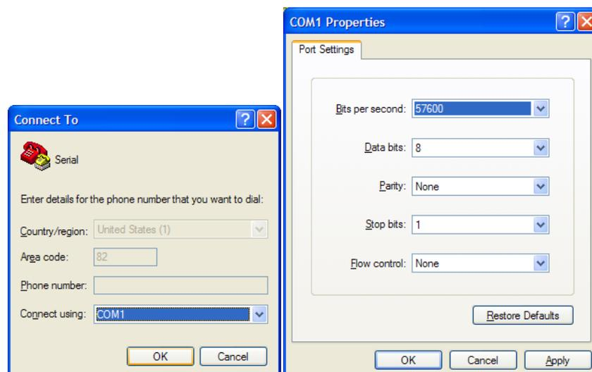
Figure 17. Serial Terminal Program configuration
