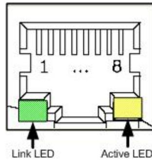
Figure 1. Pin Assignment of RJ-45 in WIZ105SR
