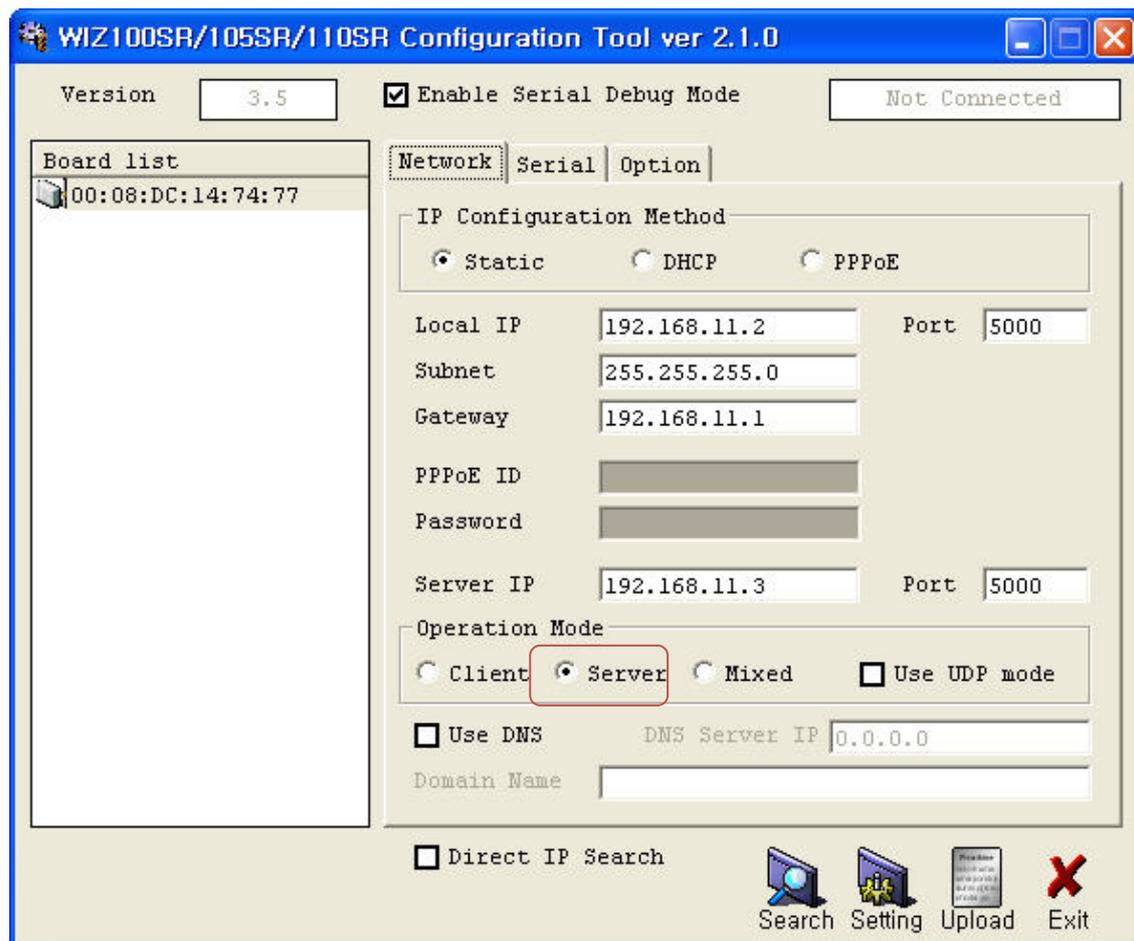
Figure 9. Operation Mode for Password Setting
