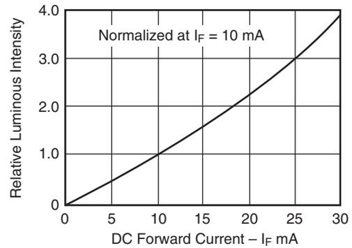
Fig. 2 Relative Luminous Intensity vs. DC Forward Current
