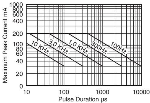
Fig. 3 Maximum Peak Current vs. Pulse Duration
