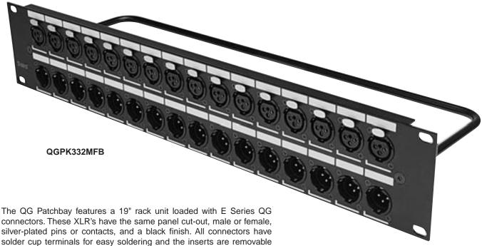
solder cup terminals for easy soldering and the inserts are removable from the back, allowing for easy changes. The one rack unit height version comes with 16 male, or 16 female, or 8 male and 8 female connectors. The two rack unit version comes with 16 male and 16 female connectors. We also offer the unit without connectors, but with the panel cut-outs already punched out. All versions have a rugged cable tie bar, which takes the weight of the cabling away from the solder connections.
