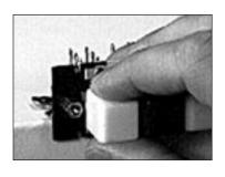
Squeeze upper and lower surfaces of pushbutton and pull free of plungers.
