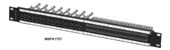
The MBPK Series combines audio and video in one convenient patchbay. The patchbay consists of 16 midsize video jacks and 48 TT bantam jacks. Options include 75 Ohm terminated or non-terminated video jacks. All TT bantam jacks have T, R, S, TN and RN solder terminals. Audio jacks have nickel-plated steel frames, gold-plated crossbar switching contacts and flared terminals for easier soldering.
