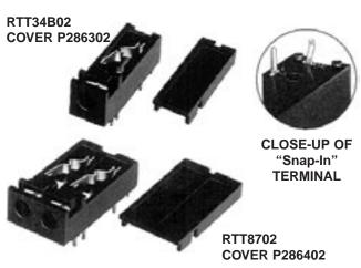
Right-angle miniature phone jacks provide low-profile packaging. Single and twin 3-conductor jacks provide plug-jack access to communication circuits for patching and/or testing. Tips and rings are shunted. These jacks mate with Switchcraft miniature TT® plugs and patch cords.
