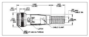
Non-reflective metal shell; 2 through 5 pins (male) or 2 through 5 contacts (female). Also 2-, 3- and 4-contact inserts with two shunted (N.C.) contacts. Efficient cable clamp and strain relief.
