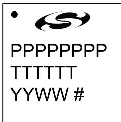
Figure 6.3. QFN28 Package Marking
