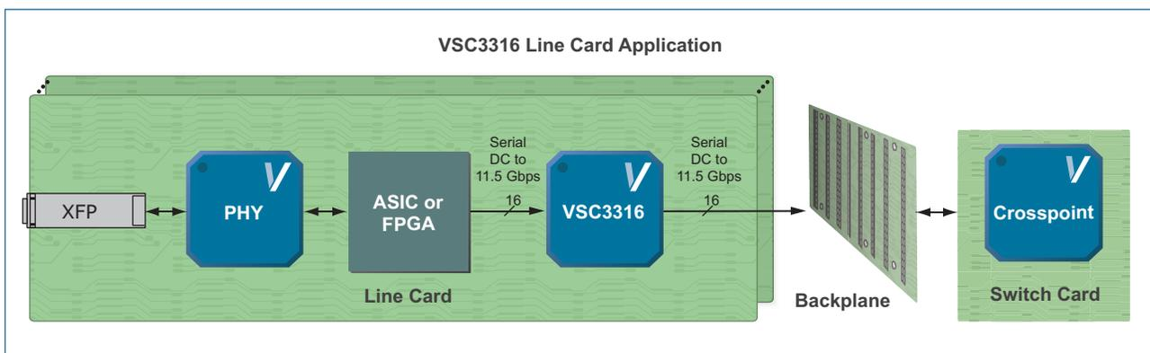
Using the VSC3316 in high-speed line cards ensures best-in-class I/O performance up to 11.5 Gbps with EQ technology to compensate for connector, backplane, and FR-4 loss.
