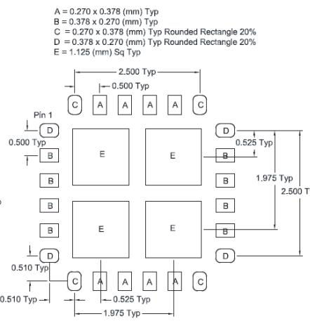
Note: Thermal vias for center slab "E" should be incorporated into the PCB design. The number and size of thermal vias will depend on the application. Example of the number and size of vias can be found on the RFMD evaluation board layout.
