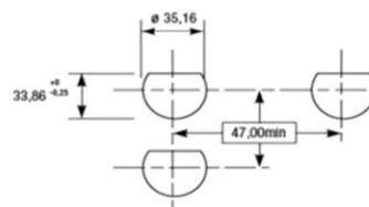
Jam nut receptacle rear panel mounting
