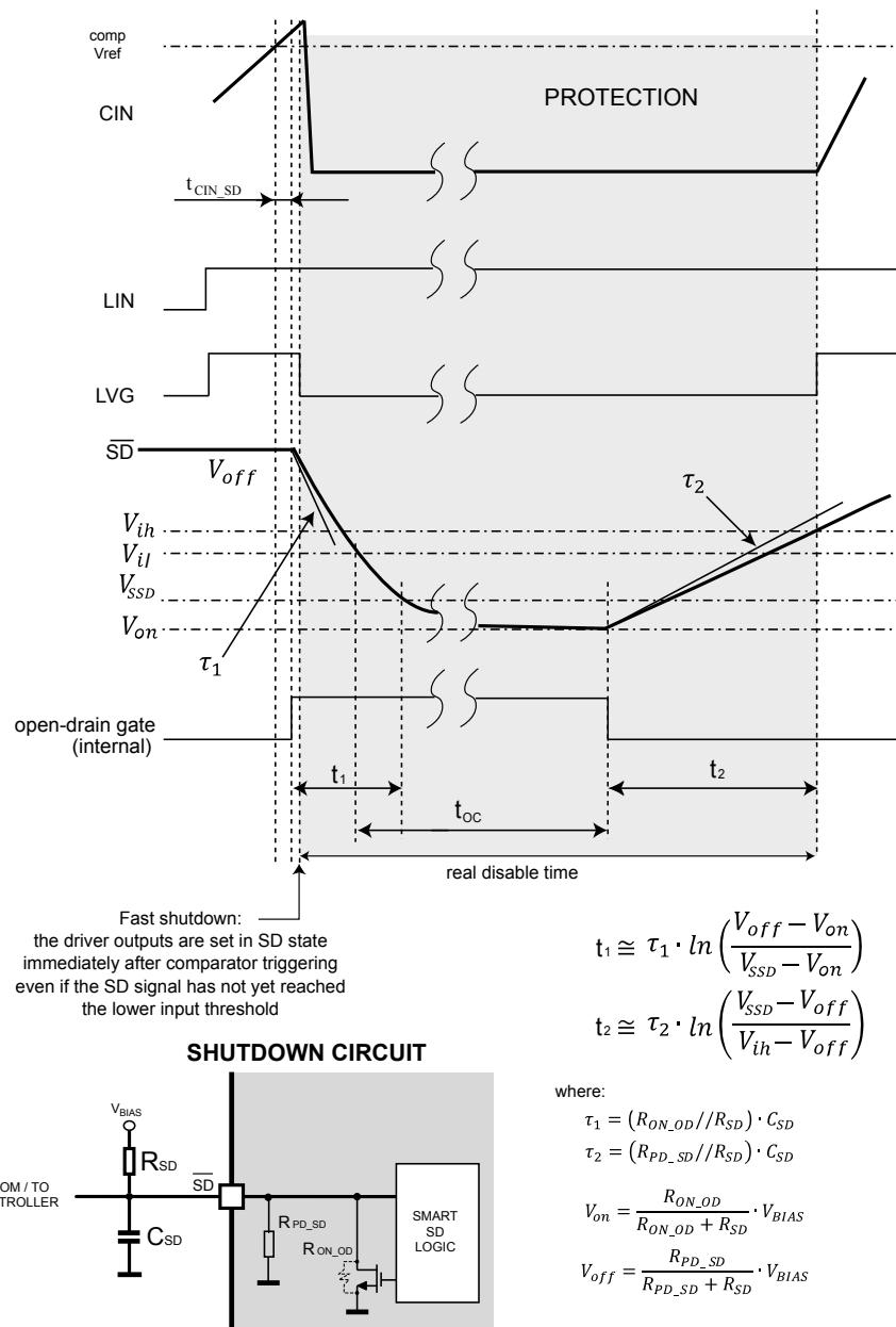
$R_{ON\_OD} = V_{OD}/5$  mA, see Table 10. Sense comparator ( $V_{CC} = 15$  V, unless otherwise is specified);
