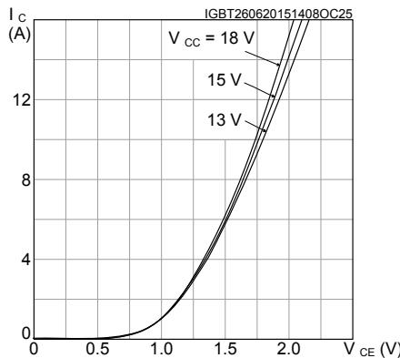
**Figure 12.  $V_{CE(sat)}$  vs collector current**
