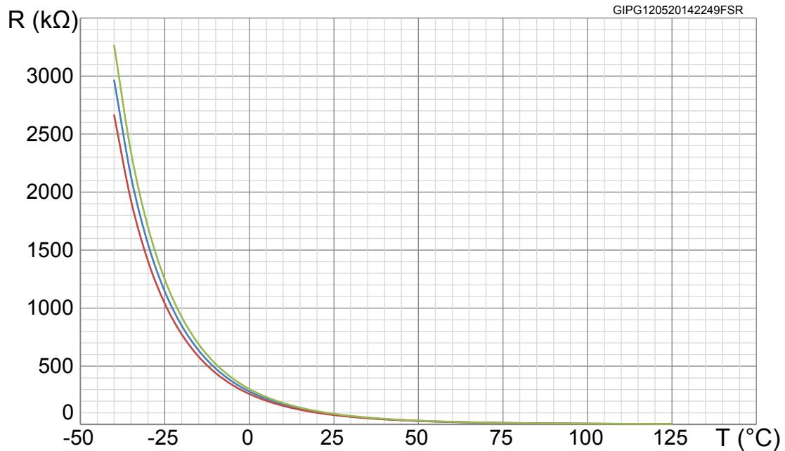
**Figure 9.** NTC resistance vs temperature - zoom
