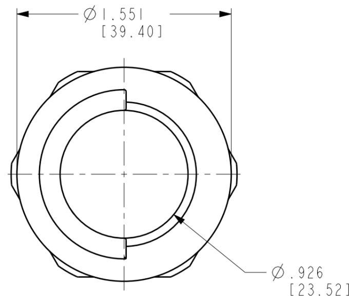
2. THIS BACKSHELL MATES WITH HDP24-18-XXP/SX-L024 AND HDP26-18-XXP/SX-L024 MAX MANUAL TORQUE 40 IN.LB.
