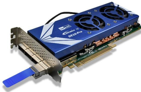
Figure 9-7 Setup QSFP28 loopback fixture
