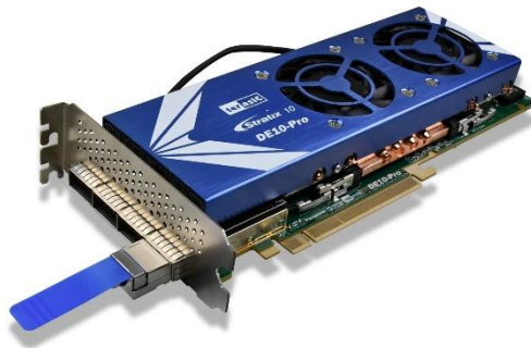
Figure 9-7 Setup QSFP28 loopback fixture
