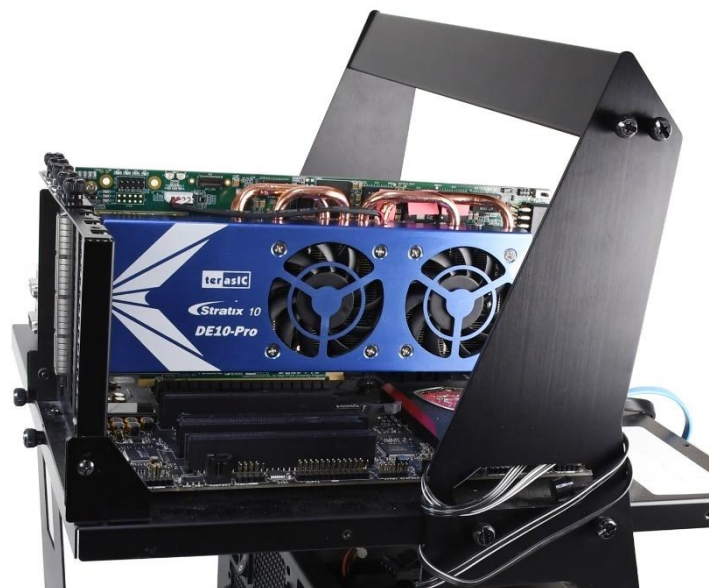
Figure 8-4 FPGA board installation on PC
