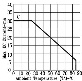
Fig5. MAX. ALLOWABLE DC CURRENT VS. AMBIENT TEMPERATURE.
