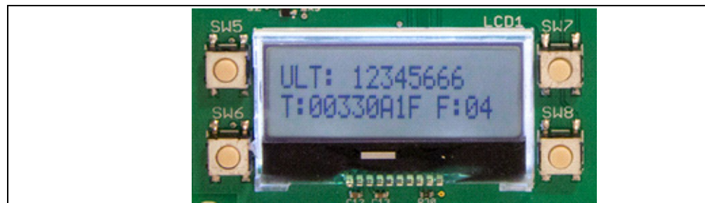
FIGURE 2-6: TYPICAL ULTIMATE KEELOQ® TRANSMISSION
