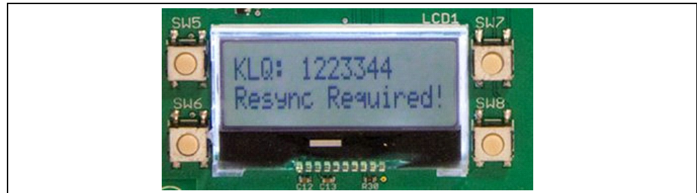
FIGURE 2-14: CLASSIC KEELOQ SYNCHRONIZATION ERROR
