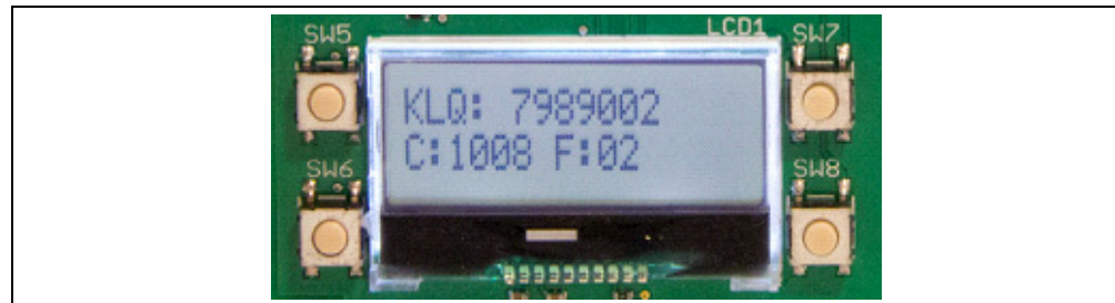
FIGURE 2-5: TYPICAL CLASSIC KEELOQ® TRANSMISSION
