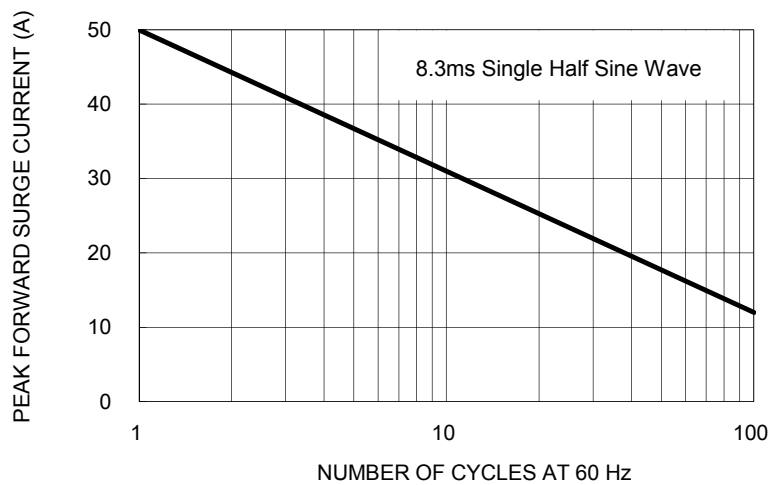
FIG. 3 MAXIMUM NON-REPETITIVE FORWARD SURGE CURRENT
