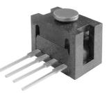
directly to the silicon-sensing element through a stainless steel plunger, with the amount of resistance changing in proportion to the amount of force applied. This change in circuit resistance results in a corresponding output level. Honeywell SIoT force sensors also deliver built-in stability and flexibility to provide enhanced performance in most applications.
