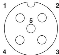
Figure 4 Pin assignment of the analog output
