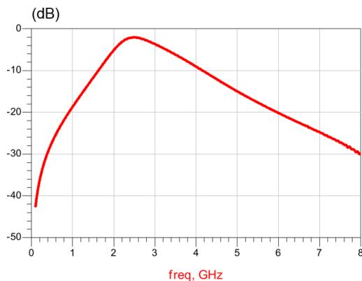
**Figure 2. Insertion loss ( $T_{amb} = 25^{\circ}\text{C}$ )**
