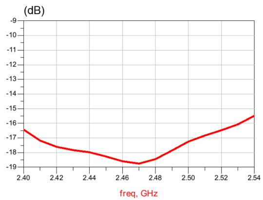
**Figure 5. Amplitude imbalance ( $T_{amb} = 25^{\circ}\text{C}$ )**
