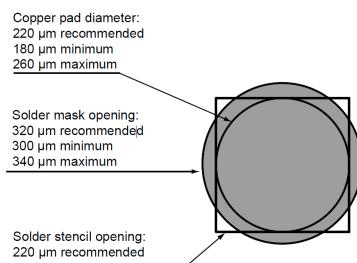
Figure 12. Footprint - solder mask defined
