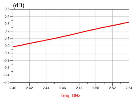
**Figure 6. Phase imbalance ( $T_{amb} = 25^{\circ}\text{C}$ )**
