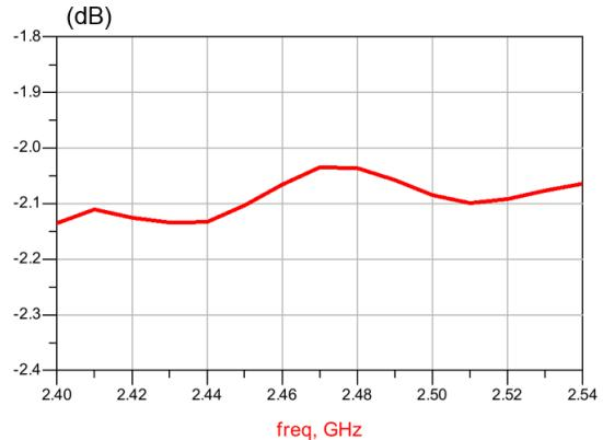
**Figure 3. Return loss on SE port ( $T_{amb} = 25^{\circ}\text{C}$ )**
