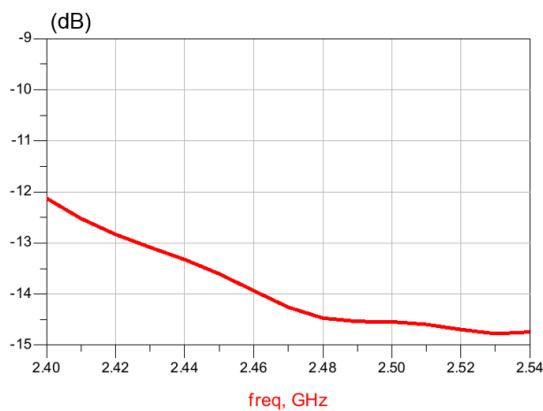
**Figure 4. Return loss on DIFF port ( $T_{amb} = 25^{\circ}\text{C}$ )**
