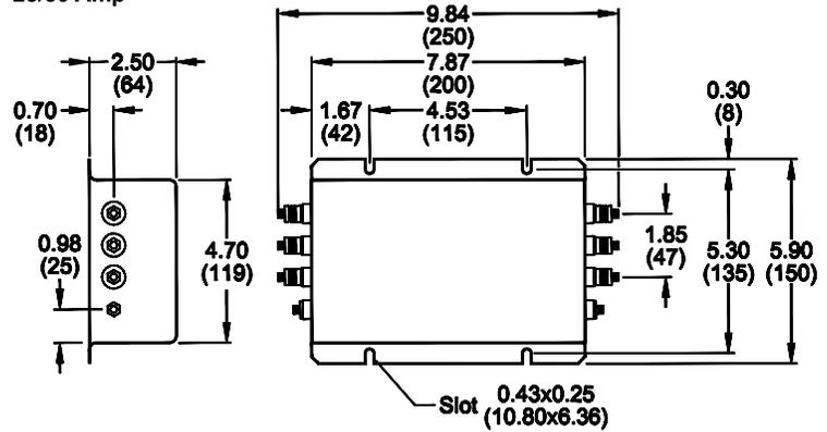
50Amp identical to 25A, except height is 3.20 (81) and bottom to center of stud is 1.25 (32)
