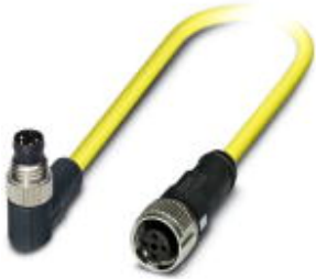
Sensor/Actuator cable, 4-position, PVC, Yellow RAL 1021, Plug angled M8, on Socket straight M12-SPEEDCON, A-coded, Cable length: 0.5 m
