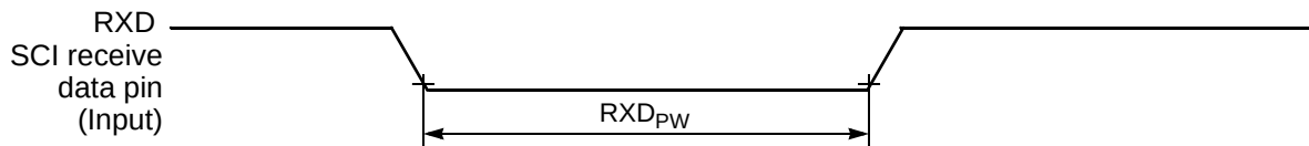
Figure 10-16 RXD Pulse Width
