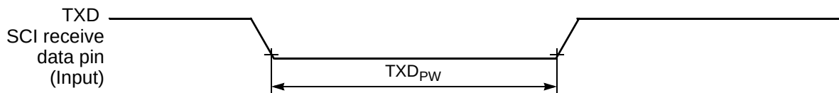
Figure 10-17 TXD Pulse Width
