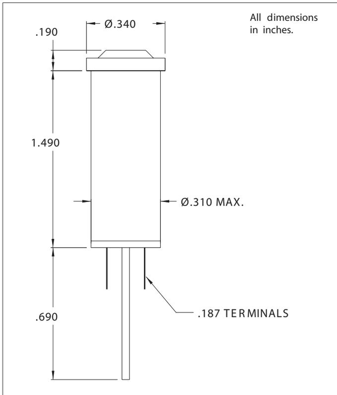
Mounting: Ø.310 MIN., supplied with push-on speednut SN1287.
