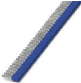
Ferrule, Dimensions according to DIN 46228-4, with color-coded plastic collars according to NF C 63-023:1994-02, for processing with the CRIMPFOX 4 in 1, Sleeve length: 8 mm, Length: 14 mm, Color: blue, Number of strips: 10, Number of sleeves per strip: 50
