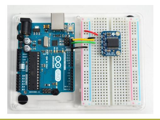
Oops i removed the Power wire from 5V to the Vin rail before taking this pic, don't forget it!
