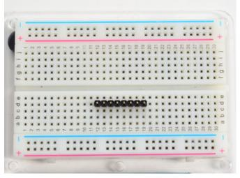
Prepare the header strip: Cut the strip to length if necessary. It will be easier to solder if you insert it into a breadboard - **long pins down**
